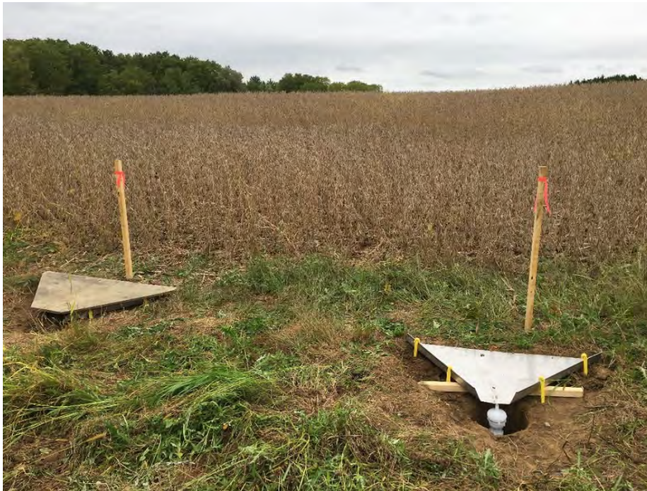
Figure A 21. Runoff trays at site DY with protective cover on (left) and off (right) with deployed sample bottle with cover designed to keep dust out of bottle when no flow occurs and to collect runoff water slowly to collect water sample over the runoff period.
