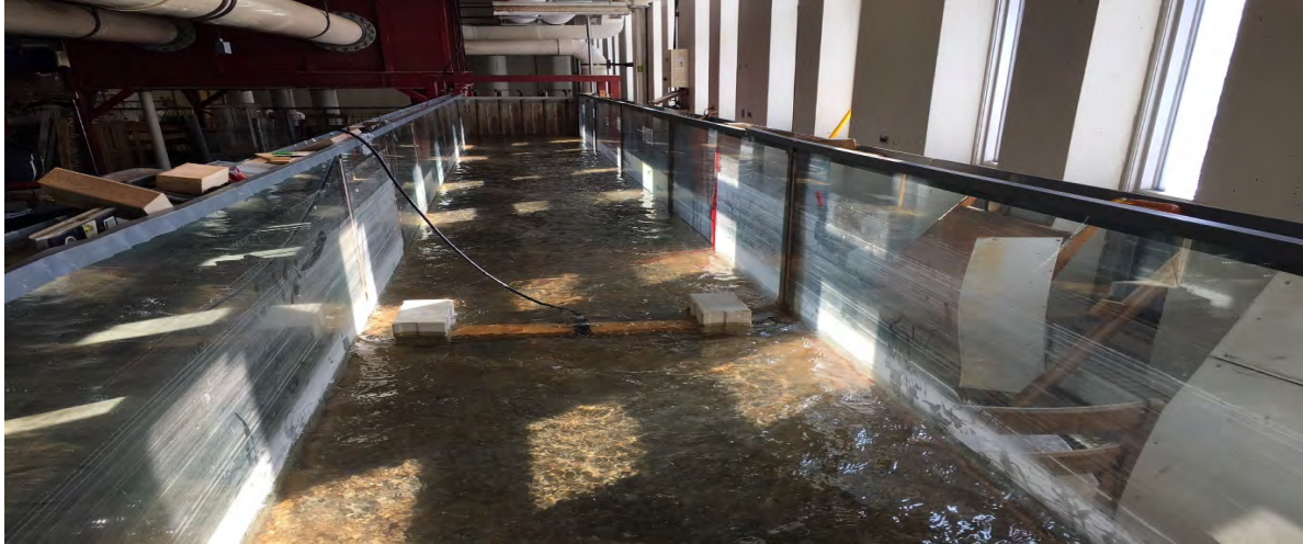
Figure A 17. Area velocity flow probe being tested for accurate calibration in a controlled flume at the Hydraulics Research and Testing Facility at the University of Manitoba prior to deployment in the field.
